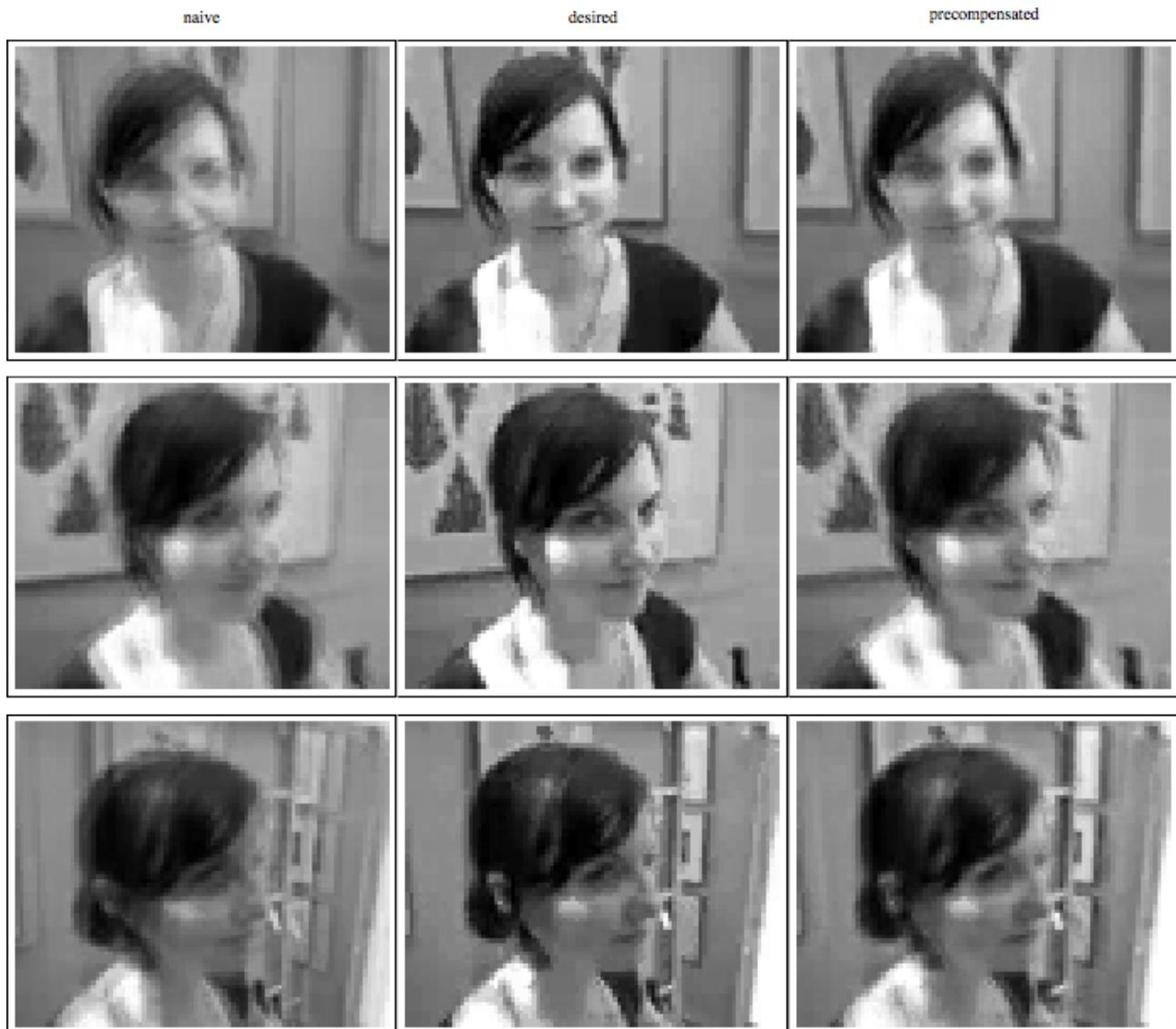
**Figure 10: A selection of monoscopic views of a simulated multiscopic display comparing crosstalk precompensation**
