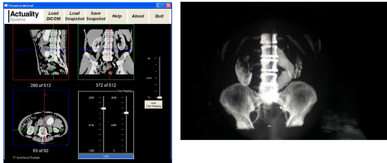
Figure 12: Perspecta Medical allows medical researchers to load standard DICOM medical data, such as CT, MR, and PET scans, for interactive viewing in 2-D and Spatial 3-D. The 2-D display presents traditional axial, coronal, and sagittal cross-sectional views of the patient. The Spatial 3-D image can be zoomed and centered by clicking on the 2-D application interface. (Public dataset available online from Philips Medical Systems.)
